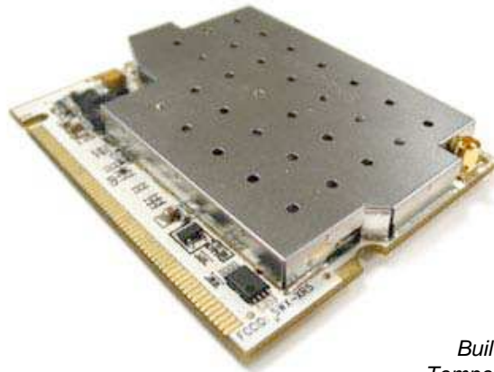
Hi-Performance PCB for Maximum RF Performance
